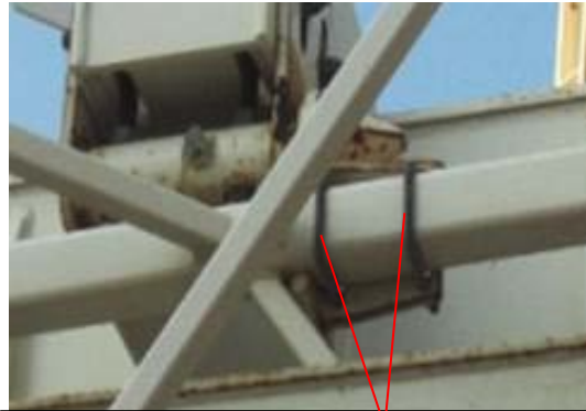
Two U-bolts securing upper attachment bracket to jib
