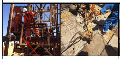
The rig floor slips under tension came free from the pad eye striking the roustabout in the face.
