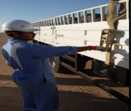
While tightening the ratchet strap, the ratchet sprung open causing him to loose his balance and fall backwards.
