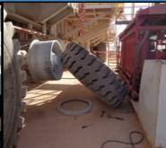
Re-inflating a tyre on the mud pump trailer when the split rims on the wheel violently exploded outwards and struck the mechanic resulting to fatality.
