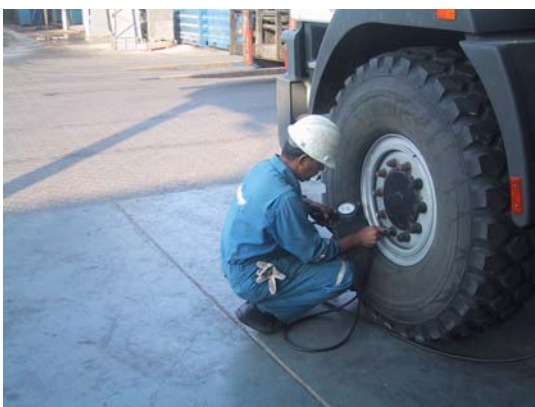
Improper position during inflation
