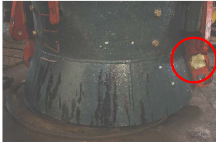
Fig 2. Position of plate at bottom of hammer
