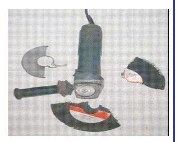
Because the disc was too big for the grinder, the worker removed the guard. He died when the disk shattered and fragments struck him in the chest and abdomen.
