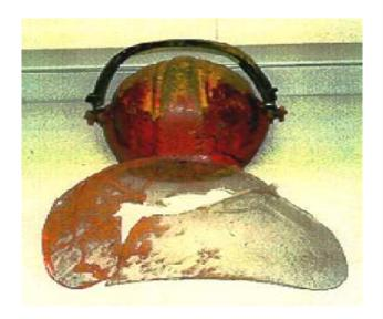
The disintegrating grinding disc penetrated the face shield, striking the worker in the face. He died on the scene. Investigation proved that the disc he used was too big for the grinder and that the guard wheel was removed to accommodate the larger disc.
