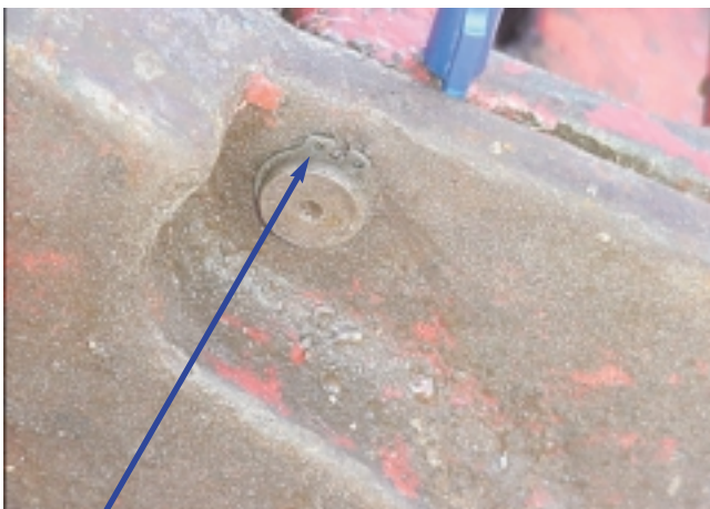
Cir-clip installed on latch pin
