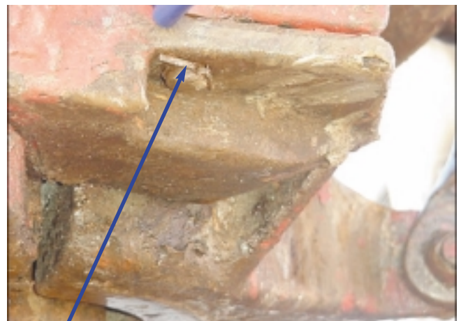
Cir-clip replaced by split pin
