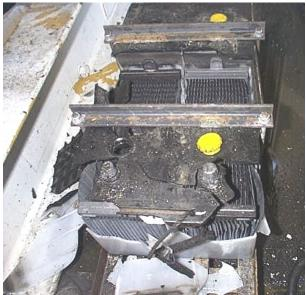
**Case # 3**: Battery shorts out, top is blown off and IP suffers acid burns **Findings**:
