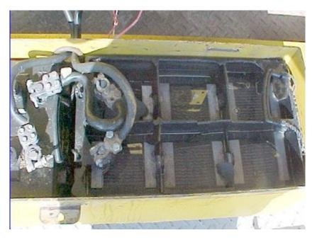
Case # 2: Battery shorts out, top is blown off and IP suffers acid burns
