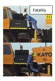
The team also identified alternative crush points on other mobile cranes including the inappropriate placement of spare wheels.
